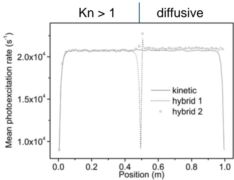
**Fig. 4** A hybrid Monte Carlo simulation that combines the kinetic equation and a fluid equation can be devised, provided a suitable interfacing between the regions is done. In the second hybrid simulation, the amount of photons escaping from the diffusive region (right) to the kinetic region (left) has been estimated using an ad hoc model.
