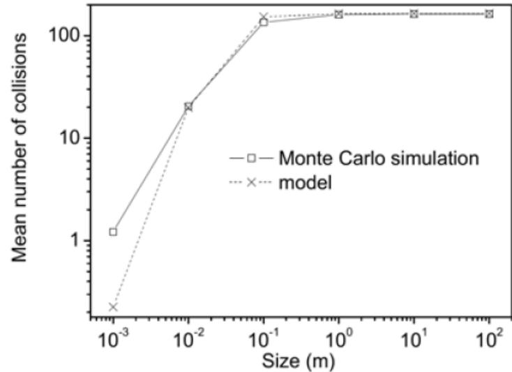
**Fig. 3** Plot of the mean number of collisions calculated using the collision estimator (Monte Carlo simulation) and the model Eq. (10). The model is in a good agreement with the simulation in highly scattering media, i.e. if the mean number of collisions is large.
