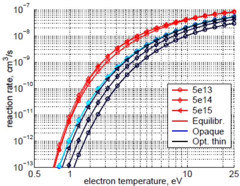
Figure 4.3: The “equilibrium” effective ionization rate, Formula (4.27), the “opaque” ionization rate and the optically thin ionization rate
