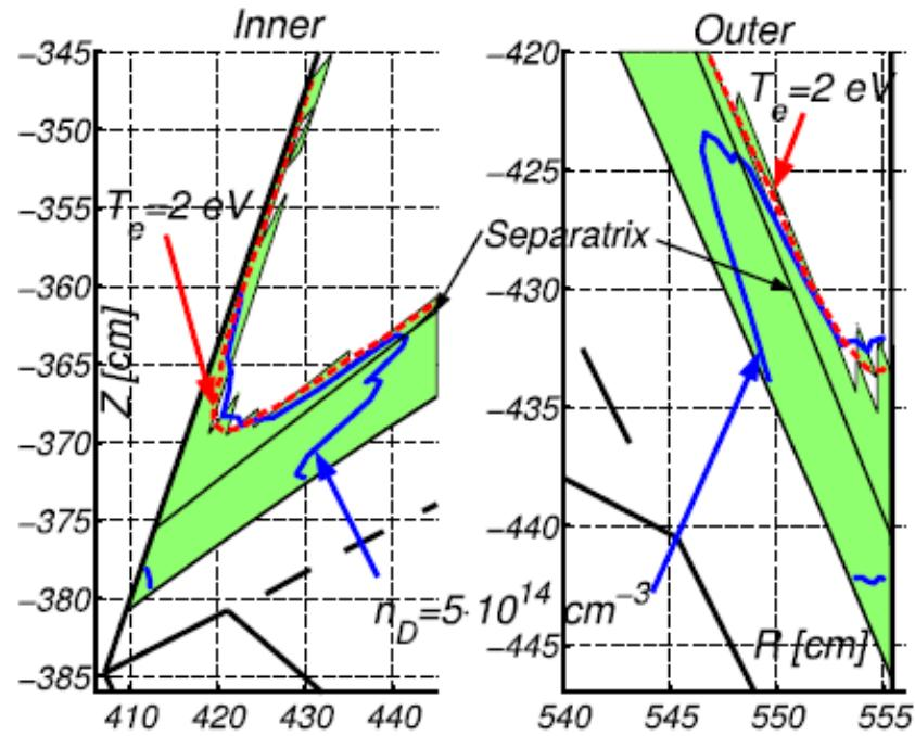
Figure 4.6: The regions in the inner and outer divertors for which the photo-induced ionization is greater than the ordinary ionization. Dashed line is the isotherm with  $T_e = 2 \text{ eV}$ , solid line is the contour of constant atom density  $n_D = 5 \cdot 10^{14} \text{ cm}^{-3}$
