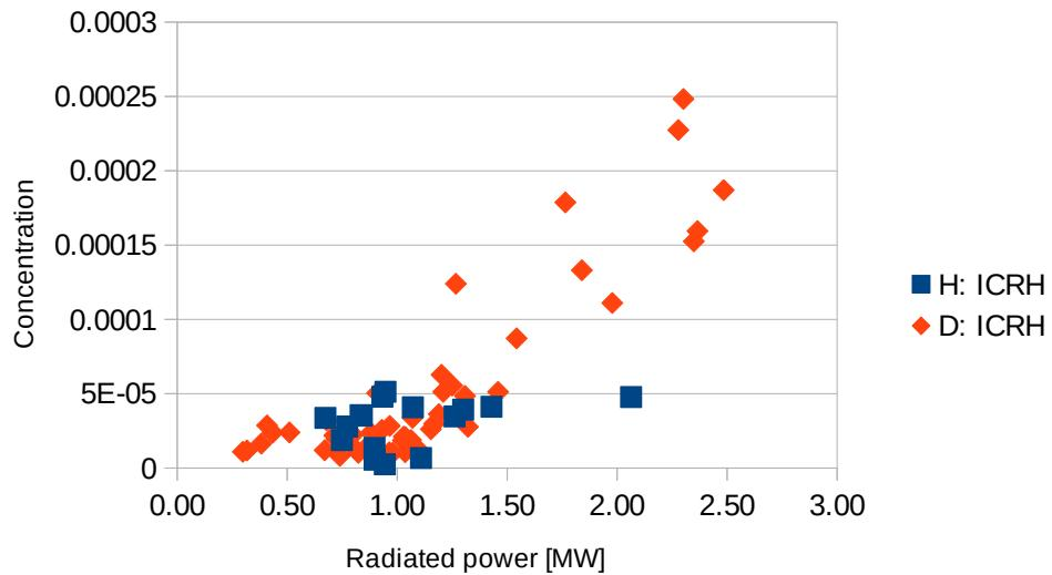
For most L-H transitions we get  $c_w$  of the order of  $10^{-4}$  for ICRH ramps and much less (an order of magnitude or more) for NBI ramps (data for D) – studies of the source of W in those two heating types
