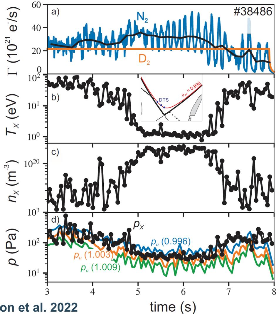
**Divertor TS measurements during a transition into the X-point radiator regime in AUG**
