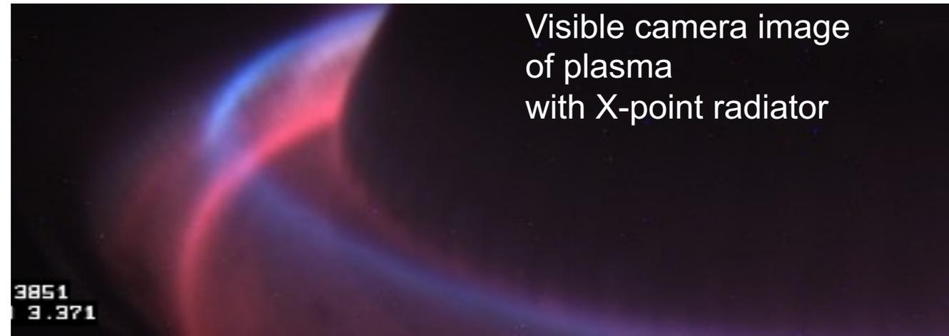
Visible camera image of plasma with X-point radiator
