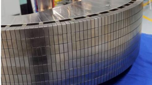
A prototype plasma-facing part of the ITER divertor. Material made of tungsten, like this, is being studied for fusion hydrogen permeation in the IAEA coordinated research project. (Photo: ITER)
