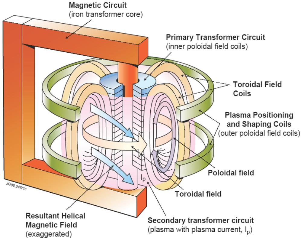
Induced poloidal magnetic field is about 1/10 of toroidal field
