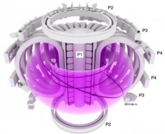
Vacuum vessel and internal divertor coils
