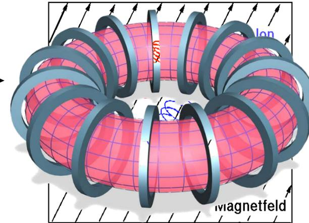
Low plasma-wall interactions (PWI) if high magnetization present, full ionisation, and no-cross field transport (ideal case).
