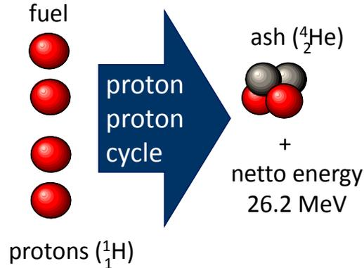
Mass defect in this reaction:  $4.8 \times 10^{-29}$  kg =>
