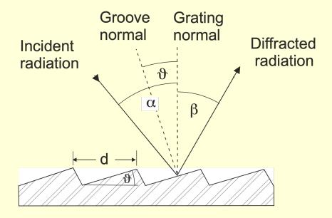
Ruled diffraction grating because of its shape diffracted power is concentrated into one direction
