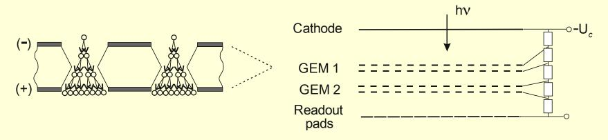
A high electric field in the bi-conical holes leads to a multiplication of the primary photoelectrons by collisional ionization
