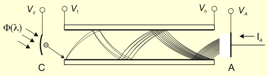
Separate photocathode can be redundant if inner wall has photo-emissive properties
