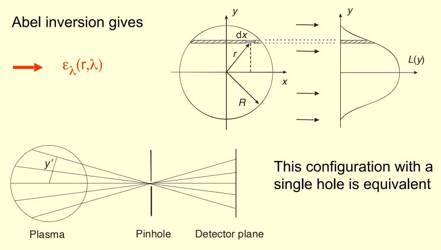
Transformation to radial symmetry is also possible for limiter tokamaks with nested eccentric circles (Shafranov shift) and and for elliptic cross-sections
