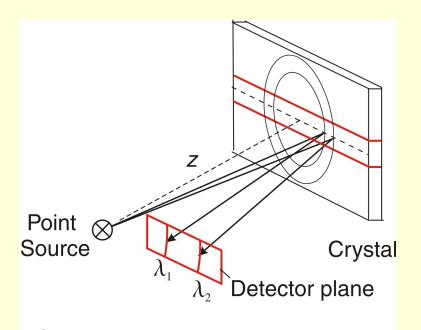
Depending on the position of the detector plane relative to the crystal the "spectral lines" are sections of a circle, an ellipse, a parabola or a hyperbola
