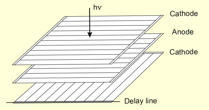
A photon produces an electron avalanche arriving on the anode, that induces an electron pulse on the cathode wires, and the difference of the arrival times at both ends yields the position
