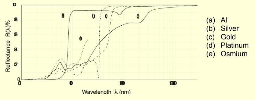
Normal incidence reflectance drops at short wavelength
