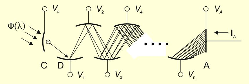
Radiant flux incident on the photocathode releases electrons; these are accelerated towards the first dynode, where they release secondary electrons, etc., till an electron avalanche arrives at the anode. This arrangemnet thus gives built-in internal amplification
