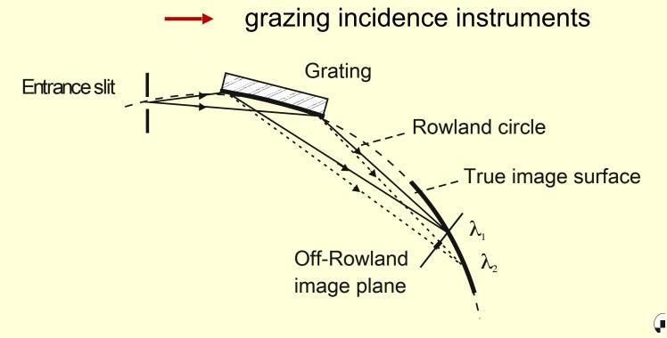
Lowest reflected wavelength for a gold coated grating is 0.54 nm for a grazing incidence angle of 2°.
