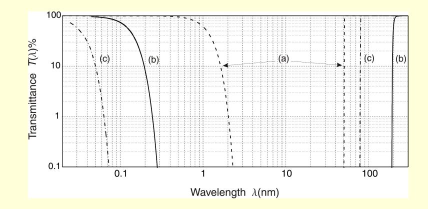
Transmission through 100 cm of gas at 101.325 kPa and 295 K: (a)He, (b) air, and (c) Ar.
