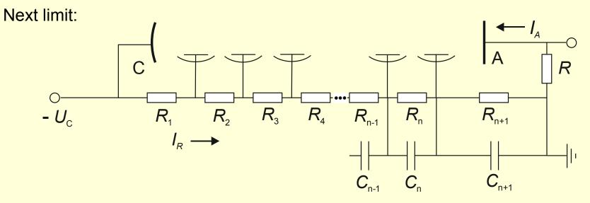
Voltage to the cathode and dynodes is supplied by a voltage divider. For high currents especially between last dynode and anode, the voltage will drop!
