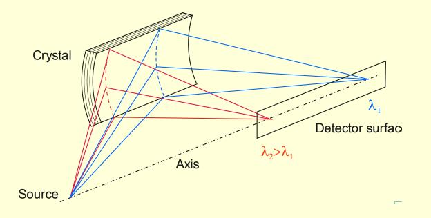
Van Hamos mount: cylindrically bent crystal, source and detector are on the cylindrical axis.
