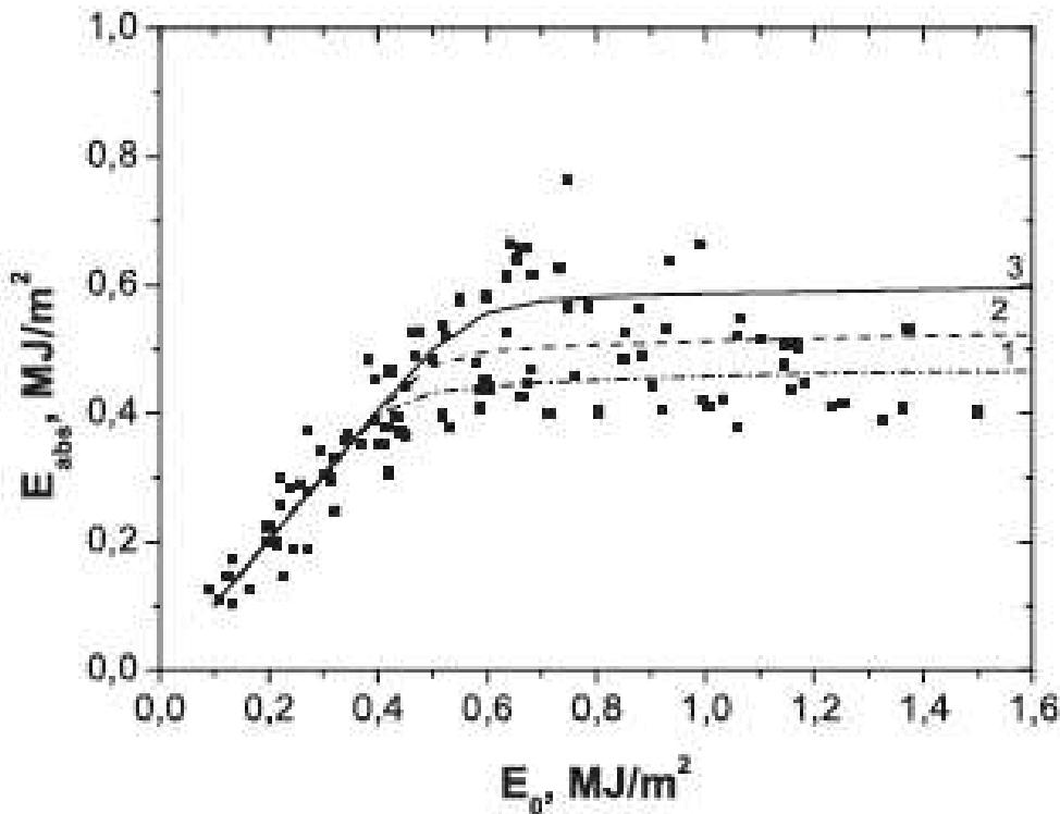
FIG. 2. The energy absorbed by the tungsten target over the energy stored in the incident plasma flow. Dots represent the experimental data obtained at MK-200 pulse plasma accelerator; curves represent the result of numerical calculations based on the second model. The first curve corresponds to  $E_{rad} = 10^{-8}$  W per evaporated particle; the second one corresponds to  $E_{rad} = 10^{-9}$  W; the third one corresponds to  $E_{rad} = 10^{-10}$  W.
