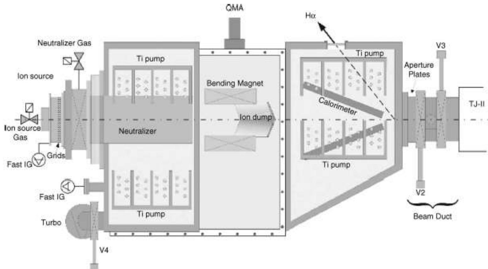
Fig. 1. Schematic of one injector with its various components and beam apertures along the beam line and duct.
