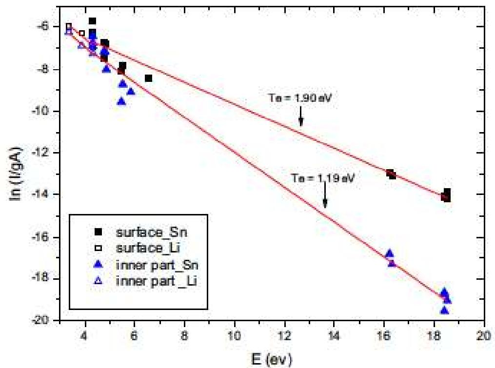
Fig. 3. The Saha-Boltzmann plot for the first laser shot of LIBS analysis. The black squares represent results from the surface of the sample and the blue squares represent the inner part of the sample (mechanically broken sample).
