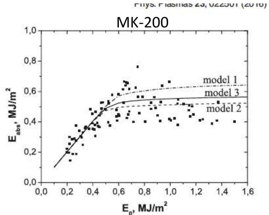
FIG. 3. The energy absorbed by the tungsten target over the energy stored in the incident plasma flow. Dots represent the experimental data obtained at MK-200 pulse plasma accelerator; curves represent the result of numerical calculations performed for three different models described.
