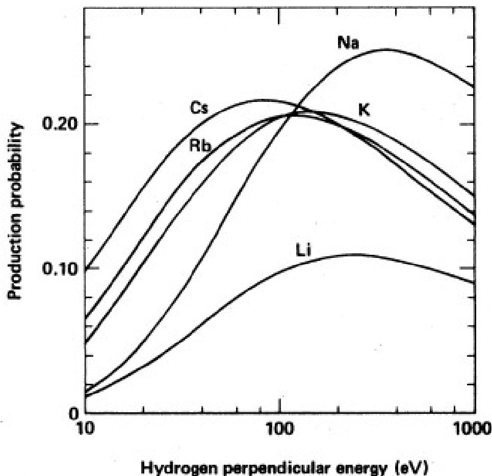
FIG. 7. The production probabilities for the different alkali metals plotted vs the perpendicular component of the hydrogen backscattered energy. For deuterium the energy scale must be doubled.
