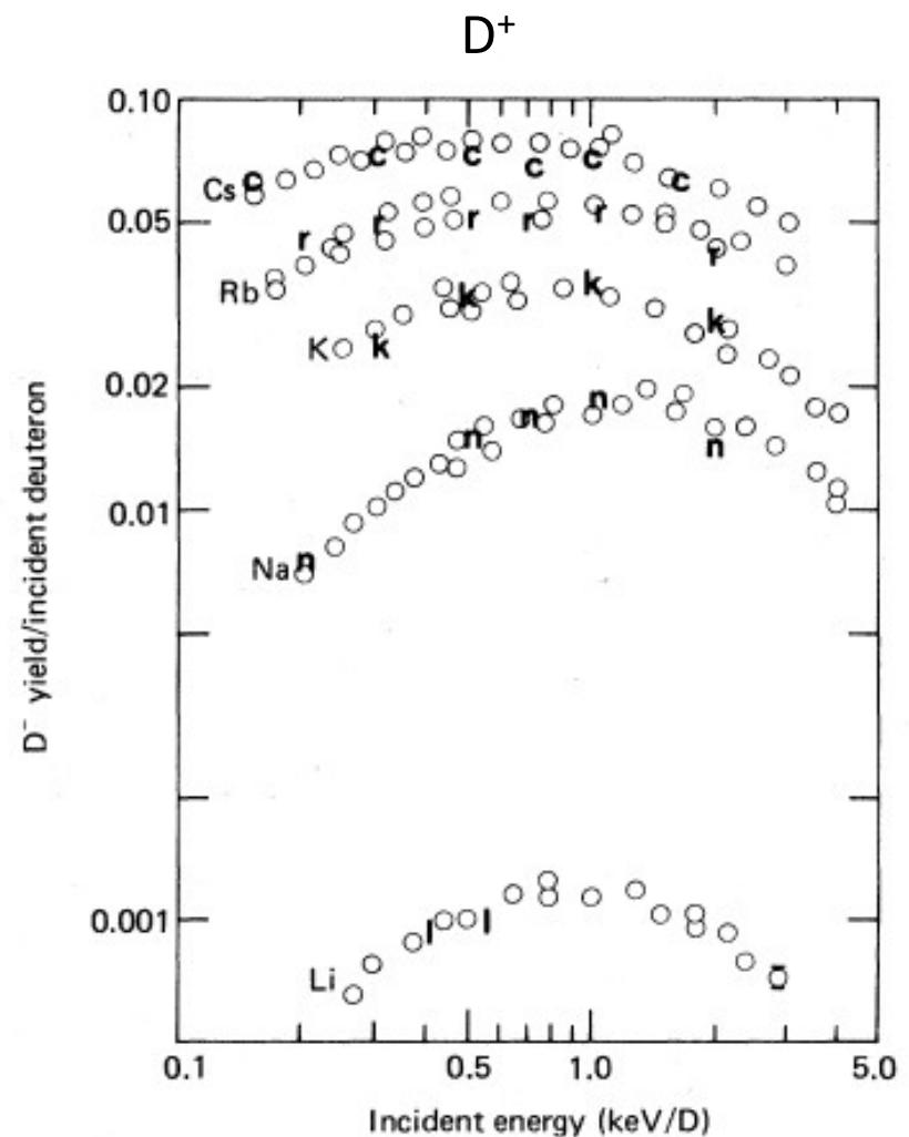
FIG. 5. Experimental NISEC values per deuteron for deuterium molecular ions incident normally upon the alkali metals vs the equivalent incident deuterium energy. The lower-case letters are the fits to the data using Eq. (7).
