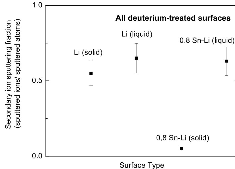
Figure 8.7. Secondary ion fraction of sputtered lithium atoms as a function of surface phase type for deuterium-treated surfaces.
