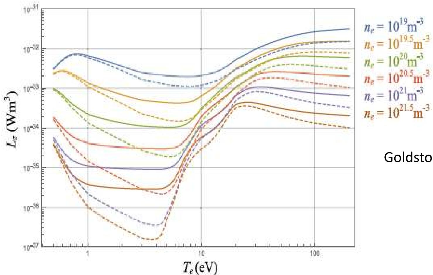
Figure 3. ADAS-based collisional radiative  $L_z$  versus  $T_e$  for  $\tau_Z = 10^{-4}$  s. Dotted lines are for radiation losses only, solid lines include power committed to ionization.
