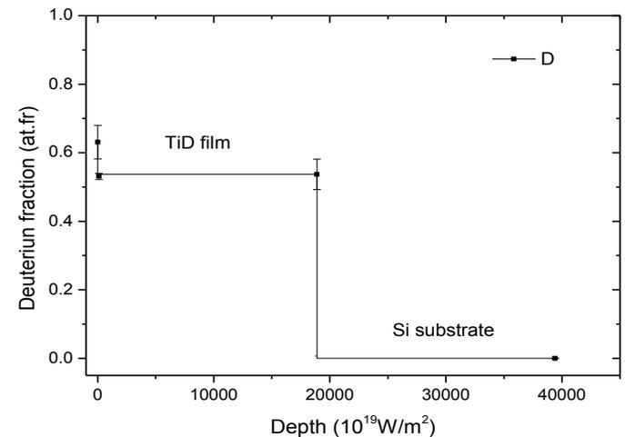
Coatings with different deuterium concentration were produced by magnetron sputtering:
