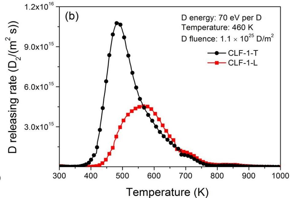
Deuterium releasing from 400 to 800 K. Unusual deuterium thermal releasing from same kind of steel sample.
