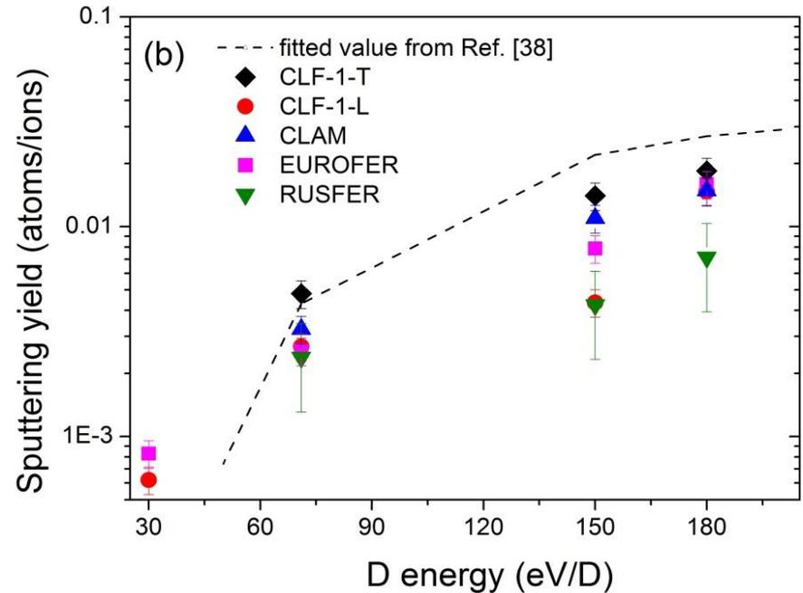
Sputtering yield of CLF-1 and EUROFER steels is lower than pure Fe, clear decreases of yield of CLF-1 steels with increasing of incident fluence. No clear saturation of yield at fluence of  $10^{25}$  D/m<sup>2</sup>.
