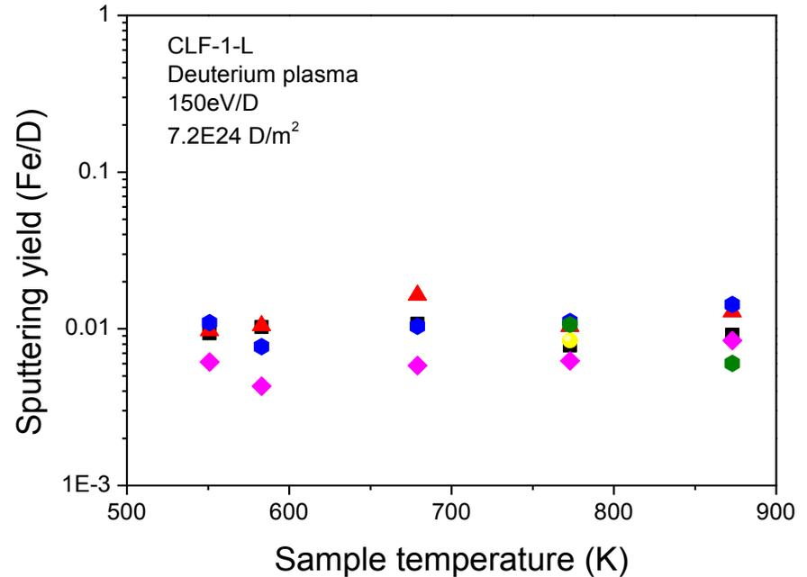
Sputtering yield of CLF-1 decreases with increasing of incident fluence, no clear saturation of yield at fluence of  $10^{25} D/m^2$ . No obvious change of sputtering yield with increase of temperature to 900 K.
