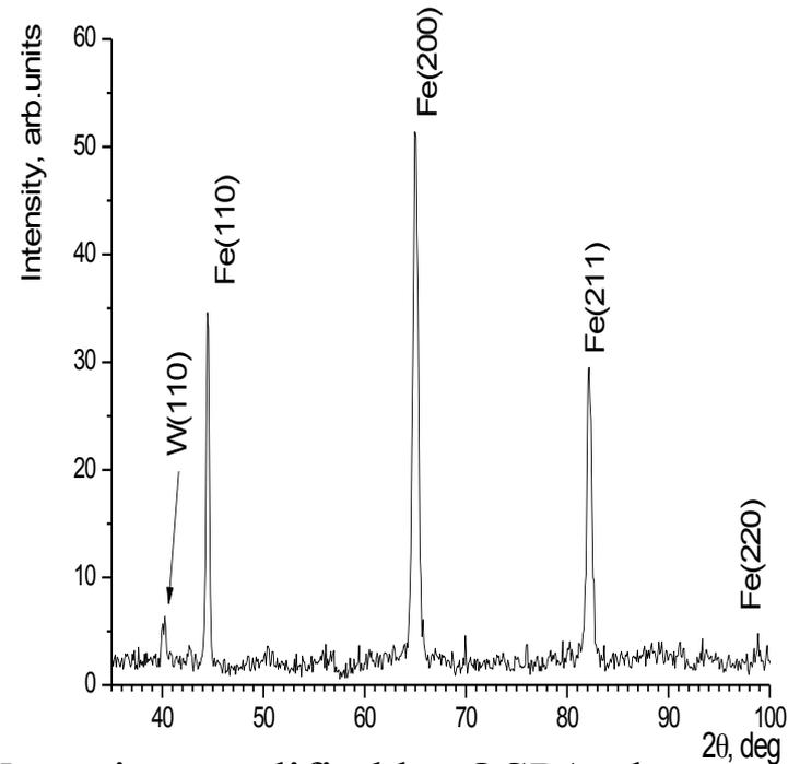
W coating modified by QSPA plasma and irradiated by Ar<sup>+</sup> beam.
