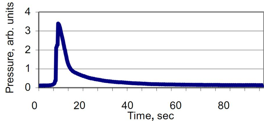
*Apparatus signal during pulsed heating of the SS sample to the temperature of 500°C*
