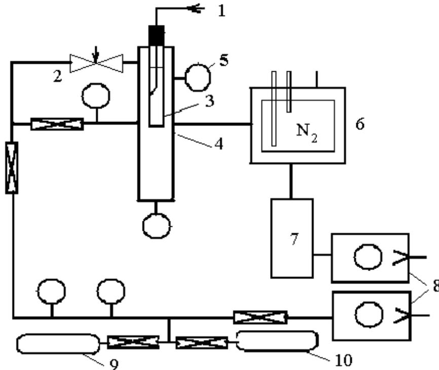
*1 – W-Re thermocouple; 2 – flow; 3 – probe; 4 – vacuum chamber; 5 – mass spectrometer; 6 – nitrogen condensation pump; 7 – diffusion pump; 8 – for-vacuum pump; 9 – hydrogen balloon; 10 – helium balloon*
