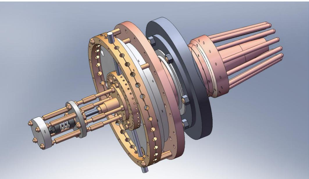
Electrode system of MPC
