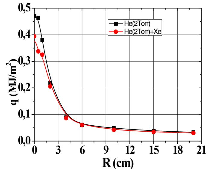
Decreasing of total energy measured by colorimeter is caused by losses to ionization of heavy impurities (Xe).
