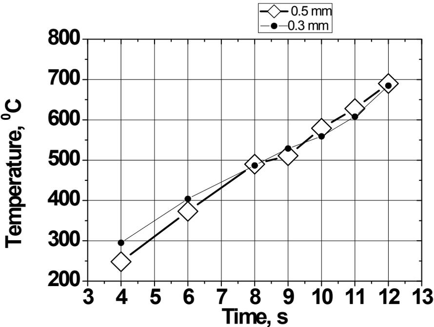
*Temperature dependence on the heating time for SS samples with thickness of 0.3 mm and 0.5 mm*
