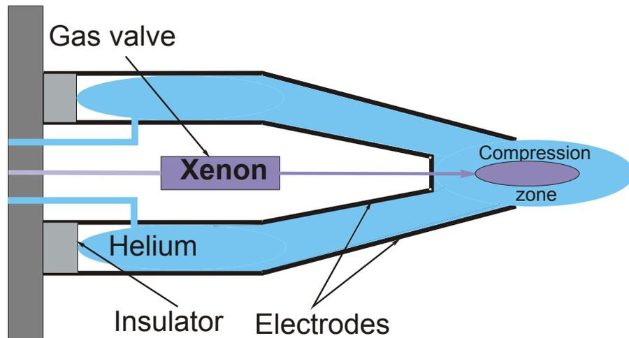
discharges in helium under different residual pressures with additional pulsed injection of Xe directly into the compression zone
