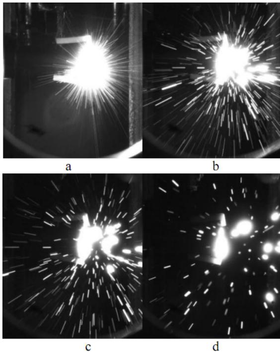
*Velocity distribution of ejected particles vs. their start time from the surface*
