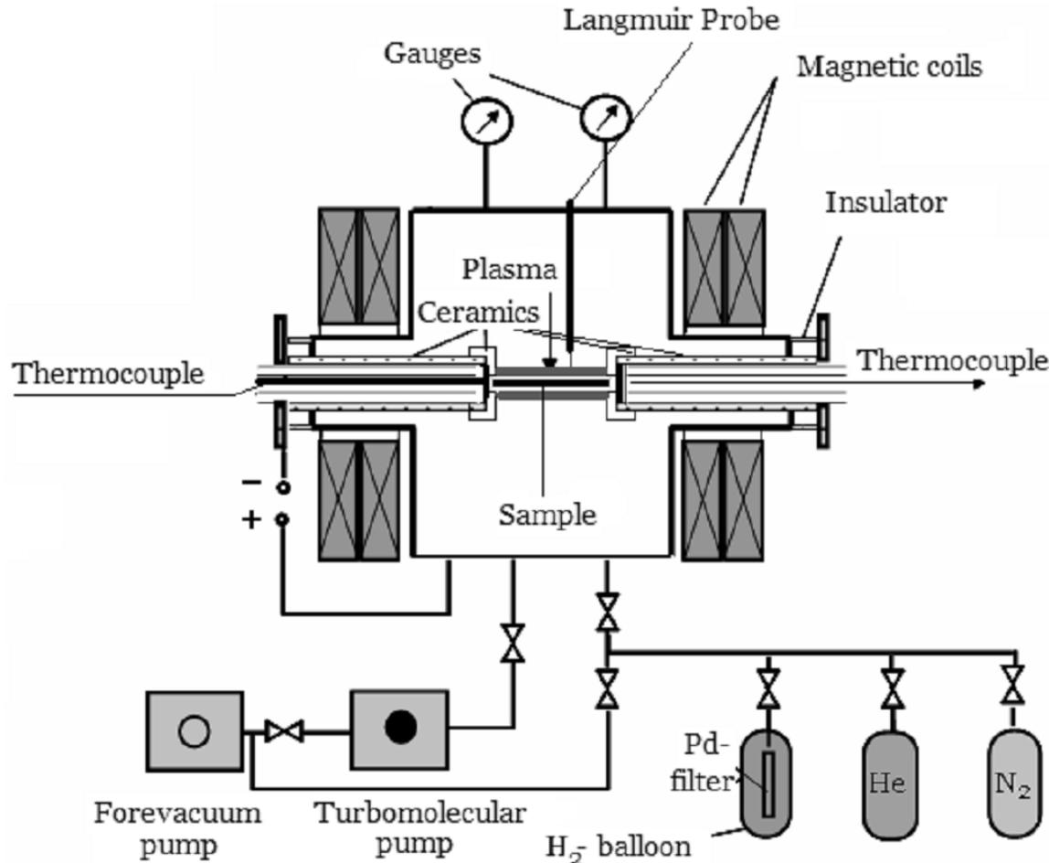
DSM-1 is device with magnetron type discharges. Two symmetrical cathodes were connected with one cylindrical cathode-sample.
