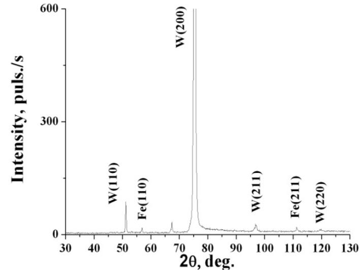
Surface coated by tungsten and exposed to
