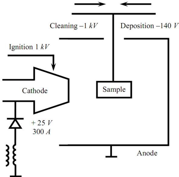
Coatings were deposited by PVD method during 3 min in argon of  $p = (4...5) \cdot 10^{-4}$  Torr.
