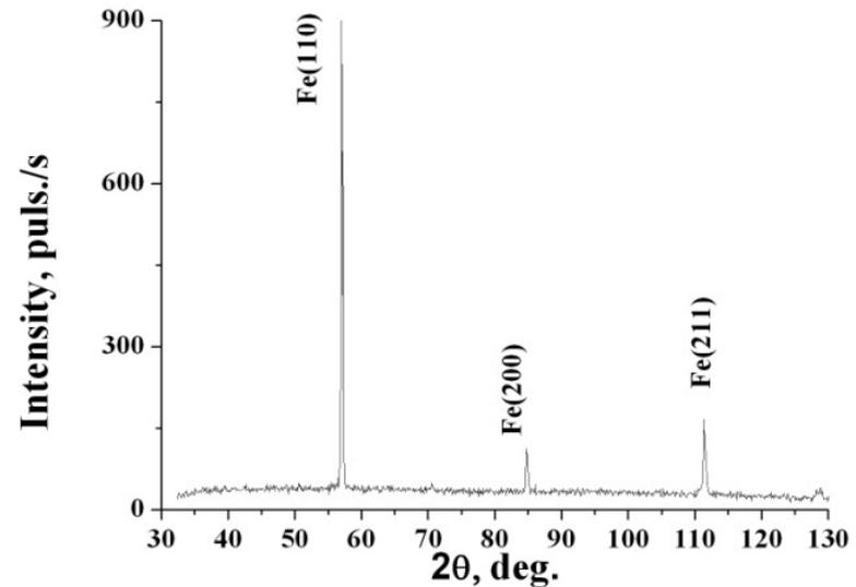
W coating modified by QSPA plasma and irradiated by Ar<sup>+</sup> beam.
