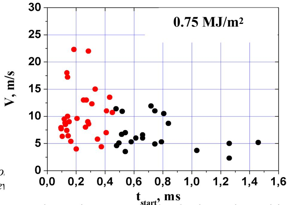
Plasma impacts with loads above the melting threshold cause the droplet/dust particles ejection from the surface of tungsten coating
