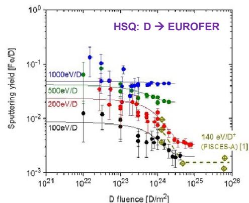
Sputtering yield of EUROFER steel by D ion irradiation with different D energies as a function of D fluence (320 K)
