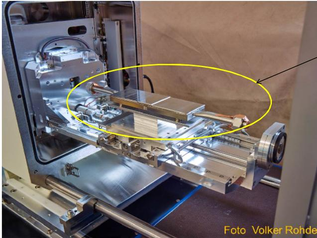
Sample mounted on heavy load sample holder for SEM
