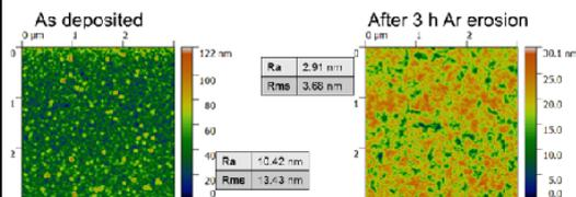
Atomic Force Microscopy of 500 nm Fe layer on Si substrate
