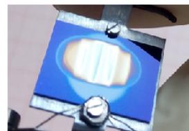
a-C:H sample eroded by inhomogeneous beam
