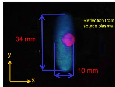
10 kV beam profile at quartz glass after dipole magnet (light blue color)
