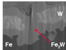
→ Fe can break through W layer at grain boundaries
