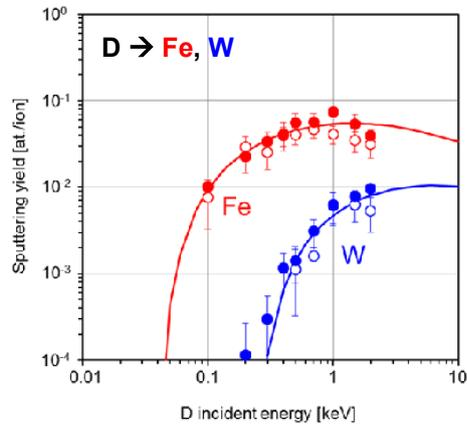
Sputtering yields of Fe and W due to D bombardment as a function of D energy.
