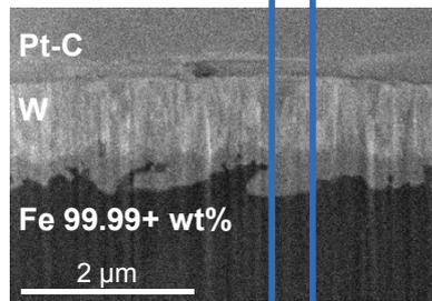
Secondary electron (SE) image of cross section produced by focussed ion beam (FIB) milling
