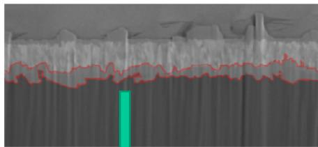
Fe<sub>2</sub>W layer (marked in red) after annealing at 1050 K
