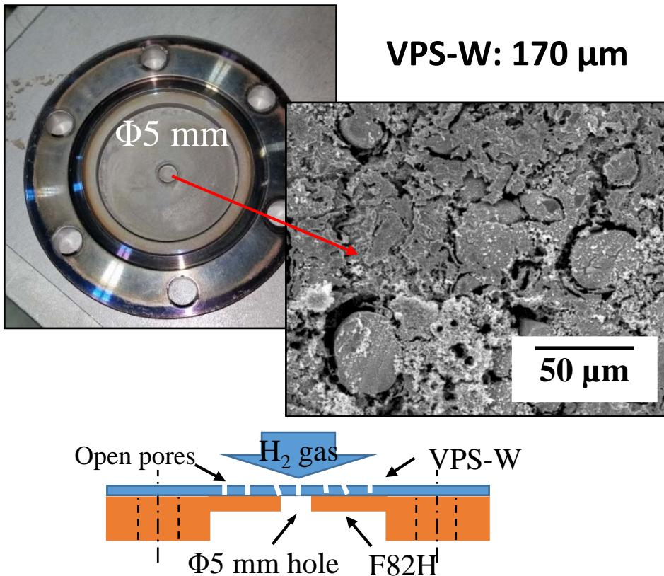
H<sub>2</sub> flows through VPS-W coatings at room temperature
