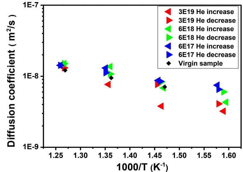
For each irradiated sample, the GDP experiments were performed from low temperature to high temperature and back to low temperature again.
