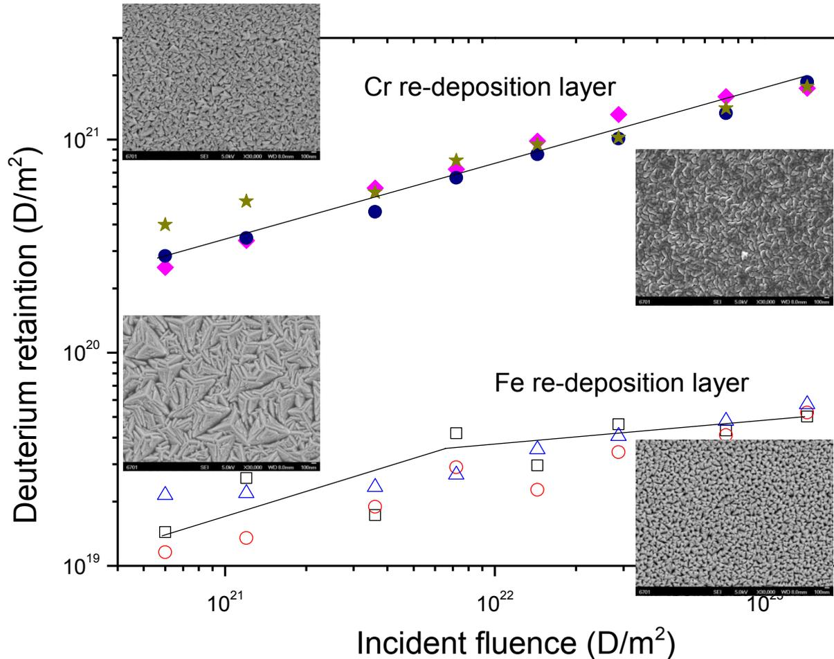
No saturation of D retention in Cr re-deposition layer
