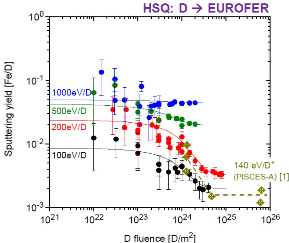
*Sputtering yield of EUROFER steel by D ion irradiation with different D energies as a function of D fluence (320 K)*
