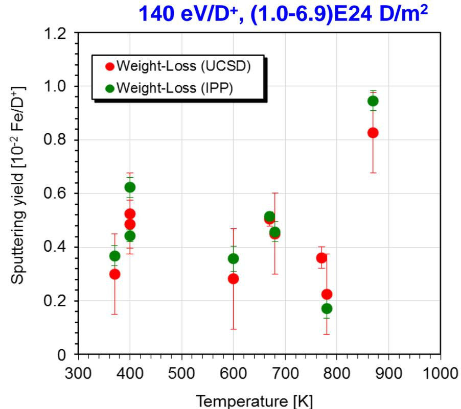
*Sputtering yield of EUROFER steel by 140 eV/D<sup>+</sup> exposure as a function of exposure temperature*
