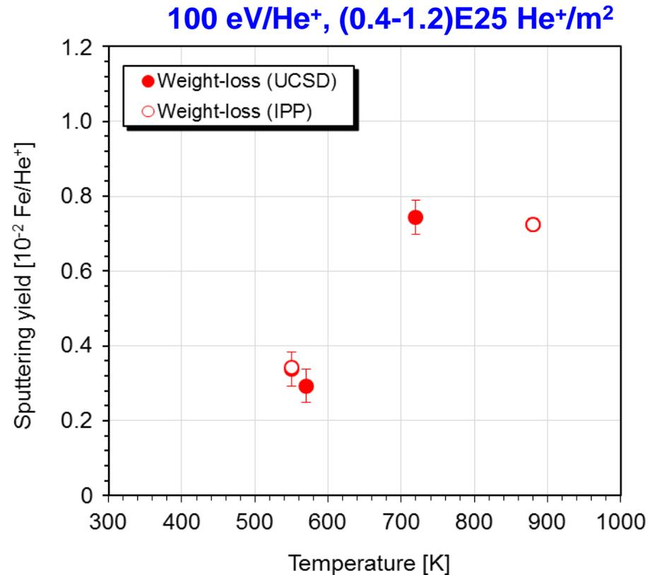
*Sputtering yield of EUROFER steel by 100 eV/He<sup>+</sup> exposure as a function of exposure temperature*
