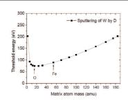
The threshold energy for sputtering of W in a Fe matrix is reduced from about 200 eV to about 100 eV.
