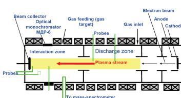
Electron beam is used to generate plasma in crossed  $E \perp B$  fields
