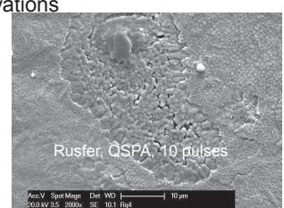
resolidified (recrystallized) layer and cracks are present
