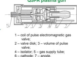
QSPA facility provides adequate pulse durations and energy densities. It is applied for erosion measurement in conditions relevant to ITER ELMs and disruptions
