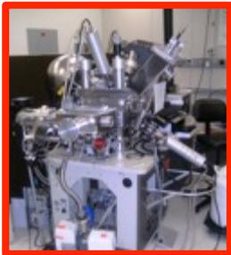
X-ray photoelectron spectroscopy (FES funded for relocation/setup)
