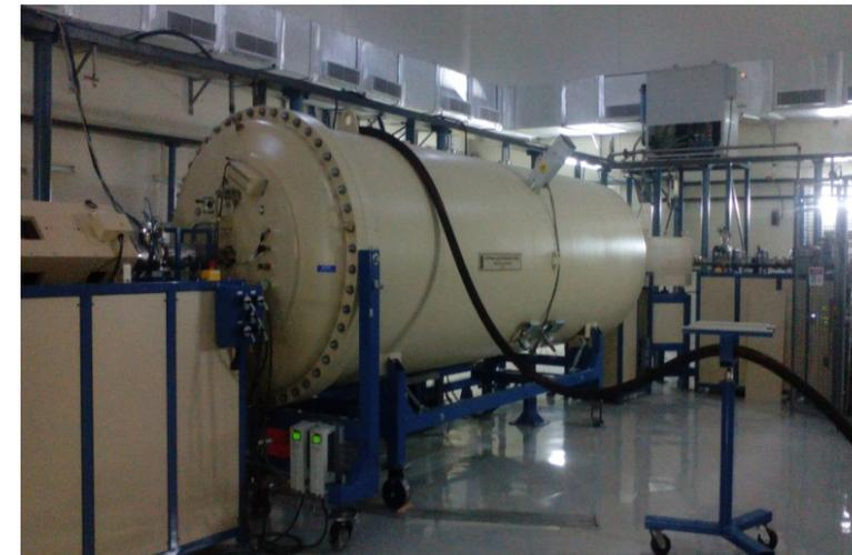
3 MV Accelerator at GG University, Bilaspur, India used for 10 MeV Boron irradiation
