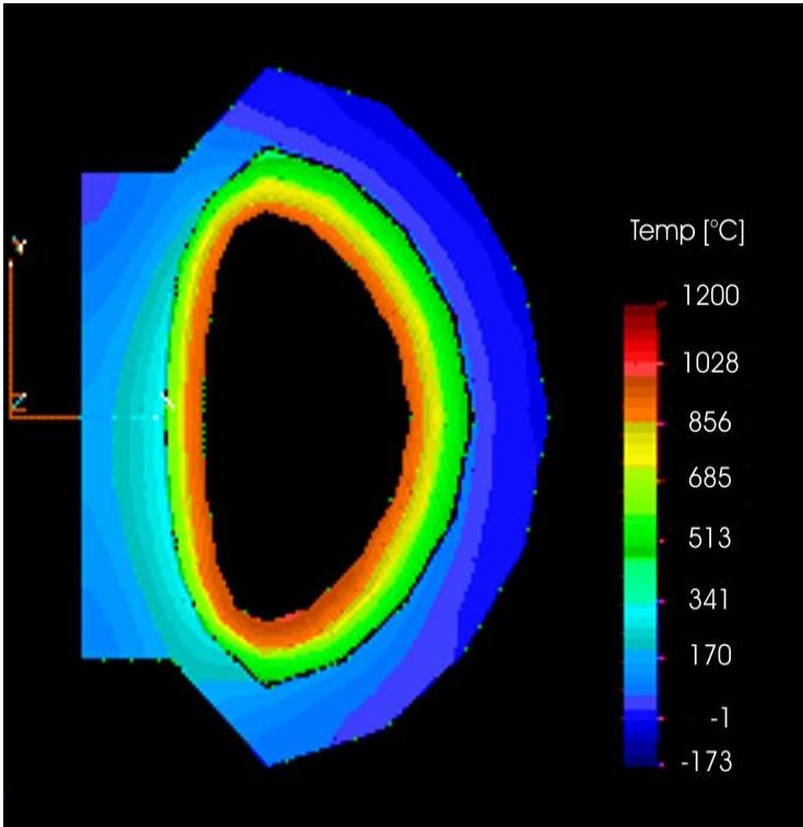
*Temperature profile in PPCS Model A, 10 days after accident with a total loss of coolant.*
