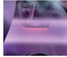
Sample for the PSI-2 side manipulator Target holder + sample in the plasma
