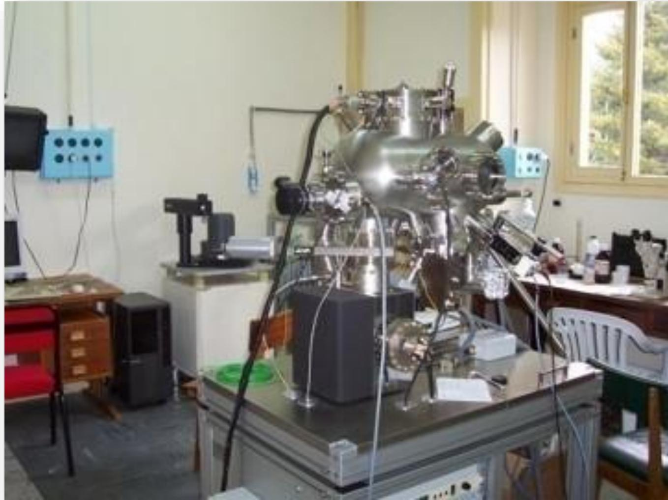
Omicron VT AFM 25 DRH microscope
