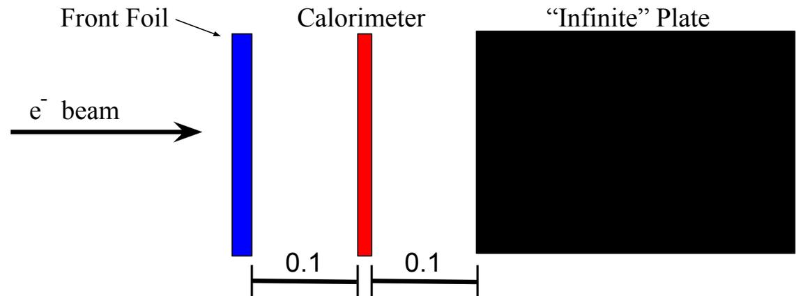
**Fig. 2.** The experimental setup of the Lockwood experiment consisting of a front foil, calorimeter foil, and “infinite” plate all of the same material and contained in vacuum.
