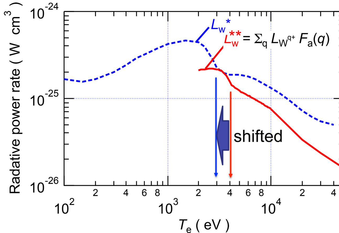
Shift of the cooling rates originates from ioniz. Eq calculation
