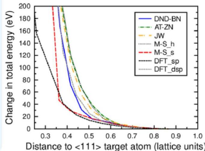
(a) Displacement in the  $\langle 111 \rangle$  direction.
