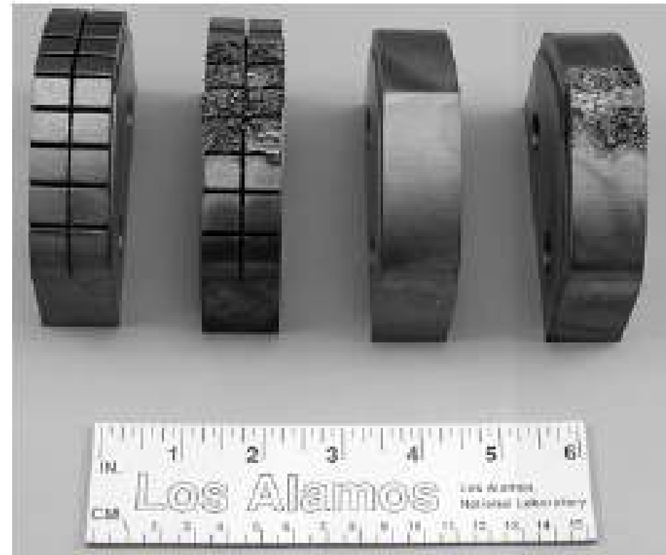
ISX-B Be limiter Tiles Used for Plasma-Spraying Tests
