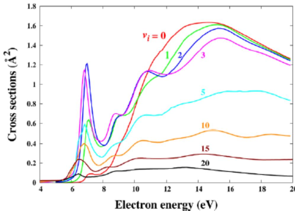
**Figure 4.** AN cross sections for processes starting from different He<sub>2</sub><sup>+</sup> vibrational levels  $v$ .
