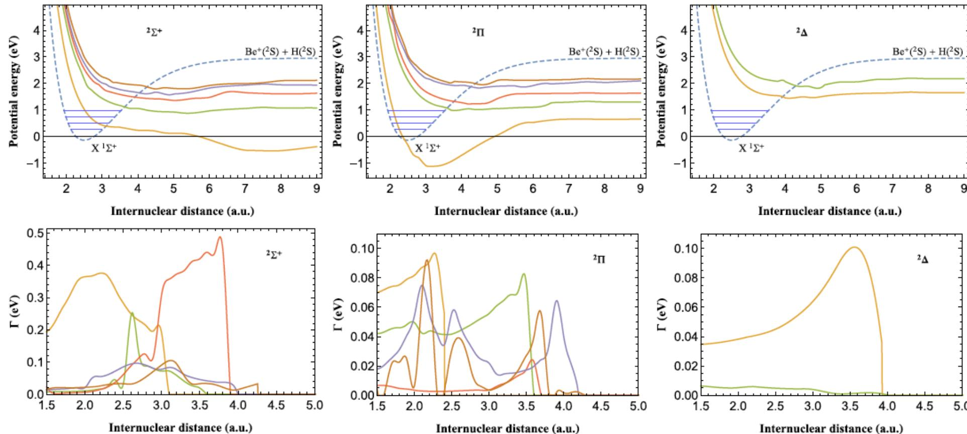
**Figure 1.** Potential energy curves (top line) and widths (bottom line) for  $\text{BeH}^{**}$  resonant states in  $^2\Sigma^+$ ,  $^2\Pi$  and  $^2\Delta$  scattering channels for  $j^+ = 0$ . Dashed line refers to potential energy curve for  $\text{BeH}^+$  ground electronic state where the first vibrational levels are marked.
