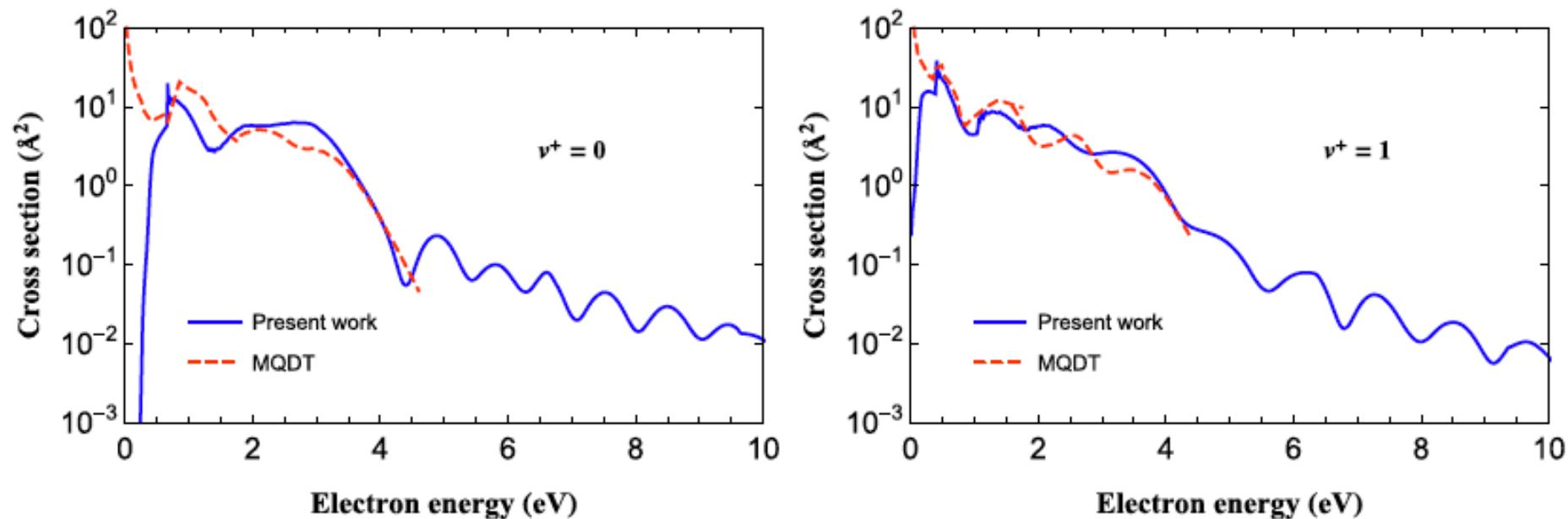
**Figure 5.** Dissociative recombination cross sections: comparison between the present calculations (full line) and MQDT/Kohn results [12] (dashed line).
