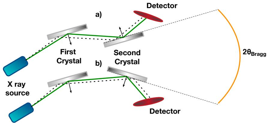
The angle difference between the two peak positions is directly correlated to the Bragg angle of the transition in question according to
