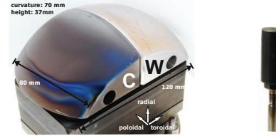
**WF<sub>6</sub> injection experiment with gas inlet and negligible limiter surface**
