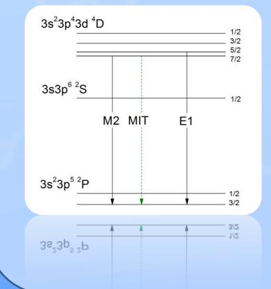
Fig. 2 Rates of the  $4D_{7/2} \rightarrow 2P_{3/2}$  transition varies along the isoelectronic sequence
